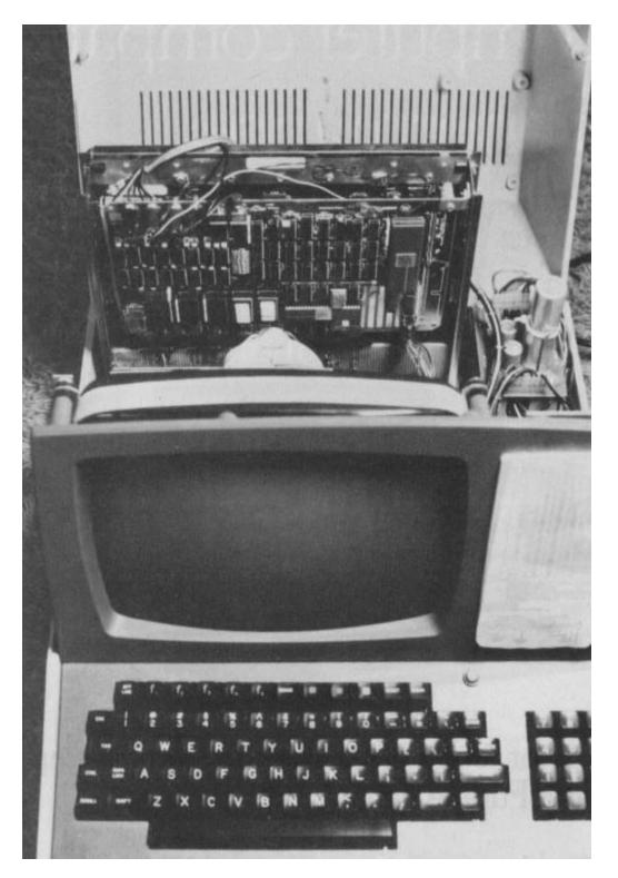
**Photo 4:** The ECB fits neatly into a Heathkit H-19 terminal. Regulated power is obtained from the H-19 through the wires in the upper left. The serial output of the terminal goes directly to the ECB, and the host port of the ECB is wired to the serial output port of the H-19. Separate holes punched in the rear chassis are for the cassette and disk I/O connectors.
