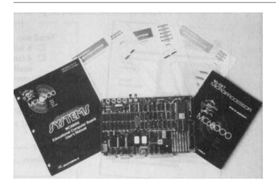
**Photo 3:** The documentation seems to dwarf the ECB. Clockwise from left are the Educational Computer Board Users' Manual, data books on the MC68230 timer, the 68000, the MC6850 serial interface adapter, and the MC68000 Programmer's Manual.
