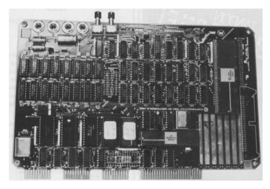
**Photo 1:** The very large integrated circuit (IC) in the upper right is the 68000. The other large IC near the wire-wrap area is the 48-pin MC68230 parallel interface/timer. The two serial interface ICs are at lower left. The edge connectors on the bottom are, from left to right, serial port 2 (host), serial port 1 (terminal), port 4 (cassette recorder), and port 3 (Centronics-type parallel printer).
